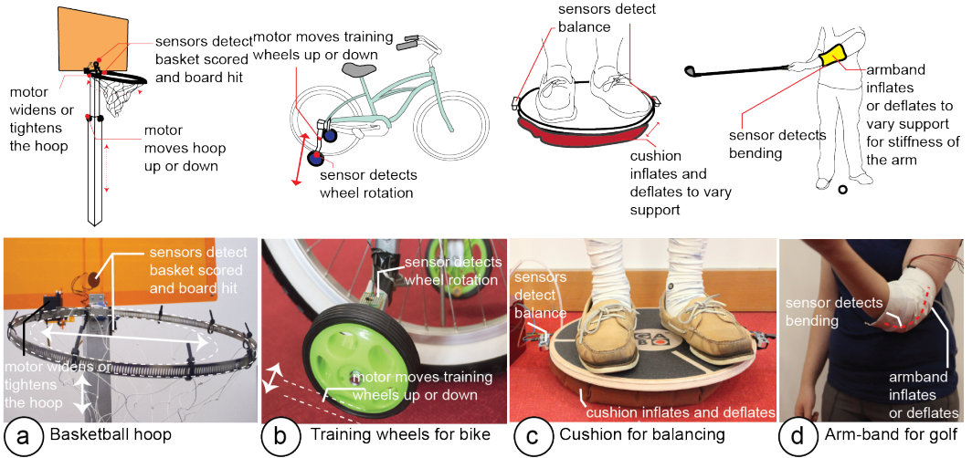
Fig. 1. Adaptive training tools adjust the task difficulty according to the learner’s current performance: (a) Adaptive basketball hoop that can be widened/tightened and raised/lowered. (b) Adaptive training wheels for a bike that can be raised/lowered. (c) Wobbleboard with inflatable/deflatable support cushion to increase/decrease stability. (d) An inflatable/deflatable golf arm band that increases/decreases restriction when bending the elbow.
